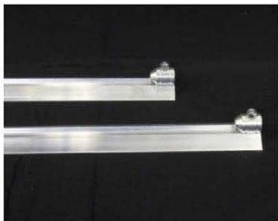
**Guidance track** is made from extruded 6061-T6 aluminum. The track is 2" wide and 7/16" tall.
